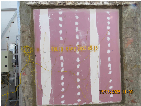
Figure 5: Un-exposed surface after the start of the test.
