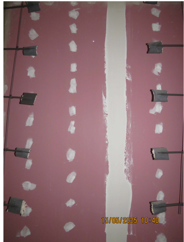
Figure 4: Exposed surface before the fire test with K-type thermocouples.
