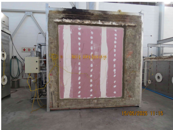
Figure 7: Un-exposed surface 15 minutes after the start of the test.
