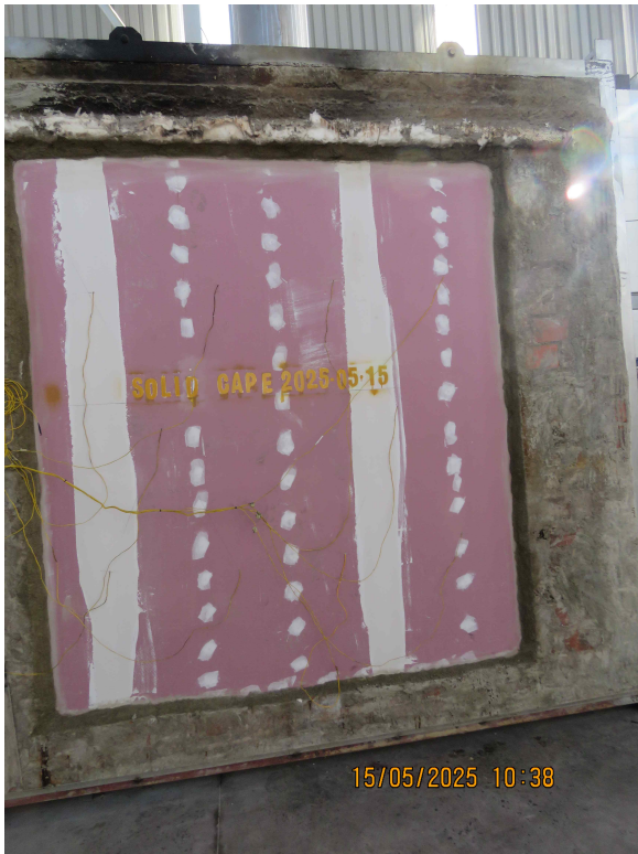
Figure 3: View of unexposed surface before the fire test.
